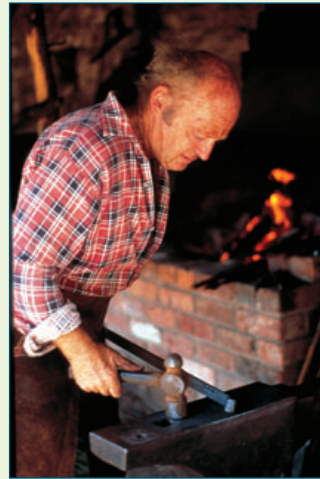
figure md.11 Shaping metal by heating and hammering.
